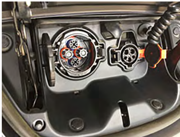
FIGURE 3 Photo shows a standard J1772 inlet on the right for use with Level 1 and Level 2 chargers; and a CHAdeMO inlet on the left. Photo from U.S. Dept. of Energy Energy, Efficiency and Renewable Energy Website: ( http://www.afdc.energy.gov/fuels/electricity_infrastructure.html ).
