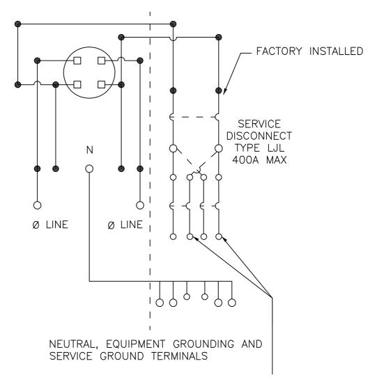
TWO BRANCH CIRCUIT BREAKERS TYPE Q2L (QBL, QDL OR QGL PREFIX) (200A MAX) MAY BE FIELD INSTALLED. ORDER ONE MOUNTING KIT CATALOG NUMBER BMK2Q400
